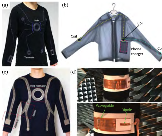
FIGURE 13. Body area networks (BANs) based on NFC: (a) Photograph of near-field-enabled long-sleeved shirt comprised of a network with a single hub and eight terminals [146]; (b) proof-of-concept NFCe jacket. The wireless signals can propagate through intricate pathways with NFC relays [147]; and based on metamaterials: (c) metamaterial textile network integrating splitters, antennas, and a ring resonator, Springer Nature 2019 [145]; (d) Wearable waveguide surface placed around the human body, IEEE 2021 [148].
